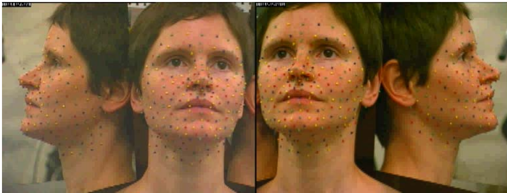
Four camera measurement setup and subject with reflexive markers (Beskow 2003)
